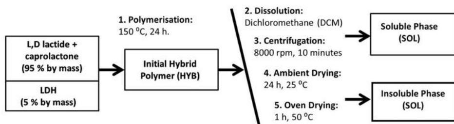
**FIGURE 1** Schematic of PN preparation process (Zhou et al., 2018)
