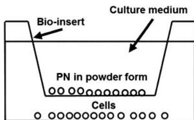
**FIGURE 2** Schematic of Saos-2 osteosarcoma cell line indirectly cultured with PNs in bio-inserts with various mass concentrations using 12-well plate
